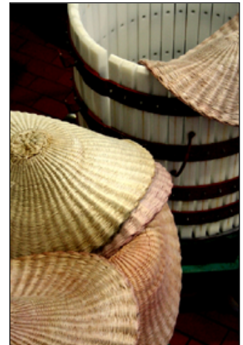
Basket press and drainage mats are handy for small, top quality parcels of reds.
